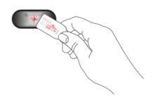
Present a user fob to the Maple antenna, located on the nearside wall at the rear of the body - Hold the fob in position until the LED stops flashing.
