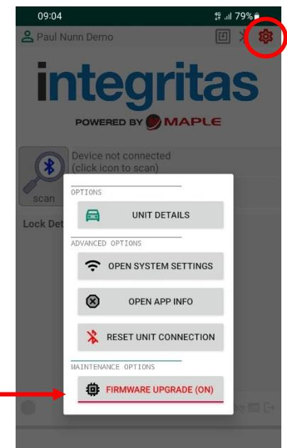
3. To perform a **Firmware Update** the **Do Not Disturb** mode must be enabled for the **Integritas App**. Follow the on-screen prompts to grant the required permissions.
